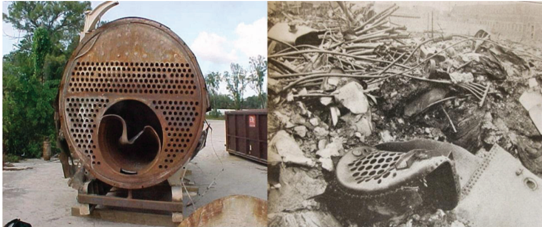
Figure 4. An “exploded” or more correctly, collapsed flue (left) is a less severe casualty than a complete failure of the pressure shell (right). Photos:
