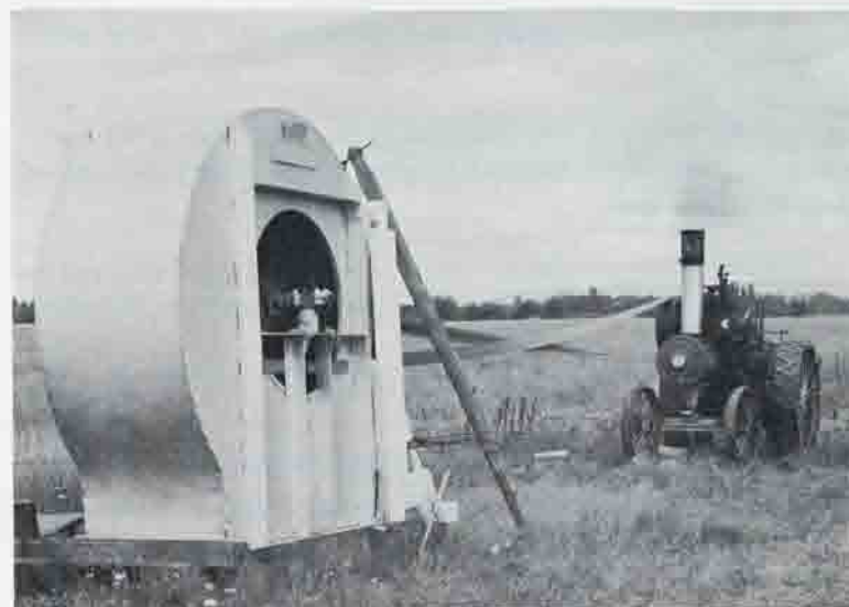
12 horse Russel. B. F. Sturtevant air circulator fan from old multi story school house. Originally powered by single cyl. steam engine. Here belted to 12 H.P. Russell 15820 14 blade rotor — 22" pulley.
