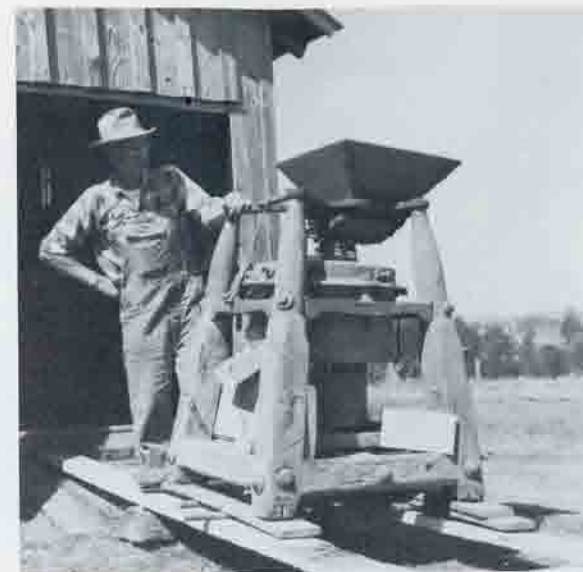
French Stone Burr grain, feed and flour grinder OWNED BY Ben O. Cole of Sublimity, Oregon. BUILT BY Nordyke and Moram, U.S.A. Age of this machine is approximately 90 years. Owned by the Cole family over 70 years.
