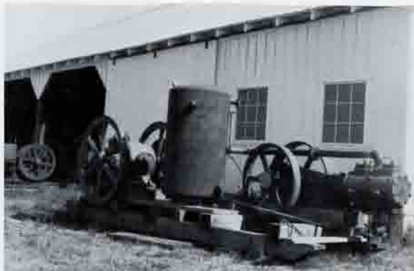
25 horse Fairbanks Morse Model Y. Hot head Diesel Engine with a 5 ft. fly wheel. The Ingersol Rand Compressor and Engine were donated to Harvey Mikkelson by Oregon Portland Cement Co. of Lake Oswego. They had a plant in Dallas and this engine was used there many years.
