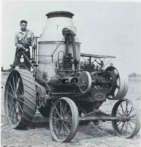
An old 1900 Westinghouse upright steamer driven by Bob Smith of Eugene has 15 horse on the drawbar. A real attraction. Owner is Willis Smith, 3636 East Main, Springfield, Oregon.
