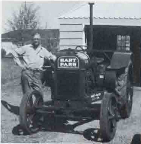
HART PARR 2 cylinder gas tractor manufactured late 1929. 12-24, is horse power rating 12 horse on Draw Bar and 24 horse on belt. It was built to burn Distilate and Kerosene. Percy L. Dezotell purchased this tractor from Mr. A. A. Neely, Deer Island, Oregon, May 31, 1965.
